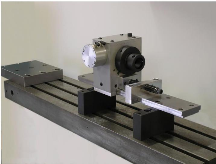
An evolution of the previous Tail Stock, the adds the ability to co-exist on the mill table with a typical mill vise. All of the controls and actuators have been moved up in the Tail Stock II to allow the head to be clamped in the mill vise.
