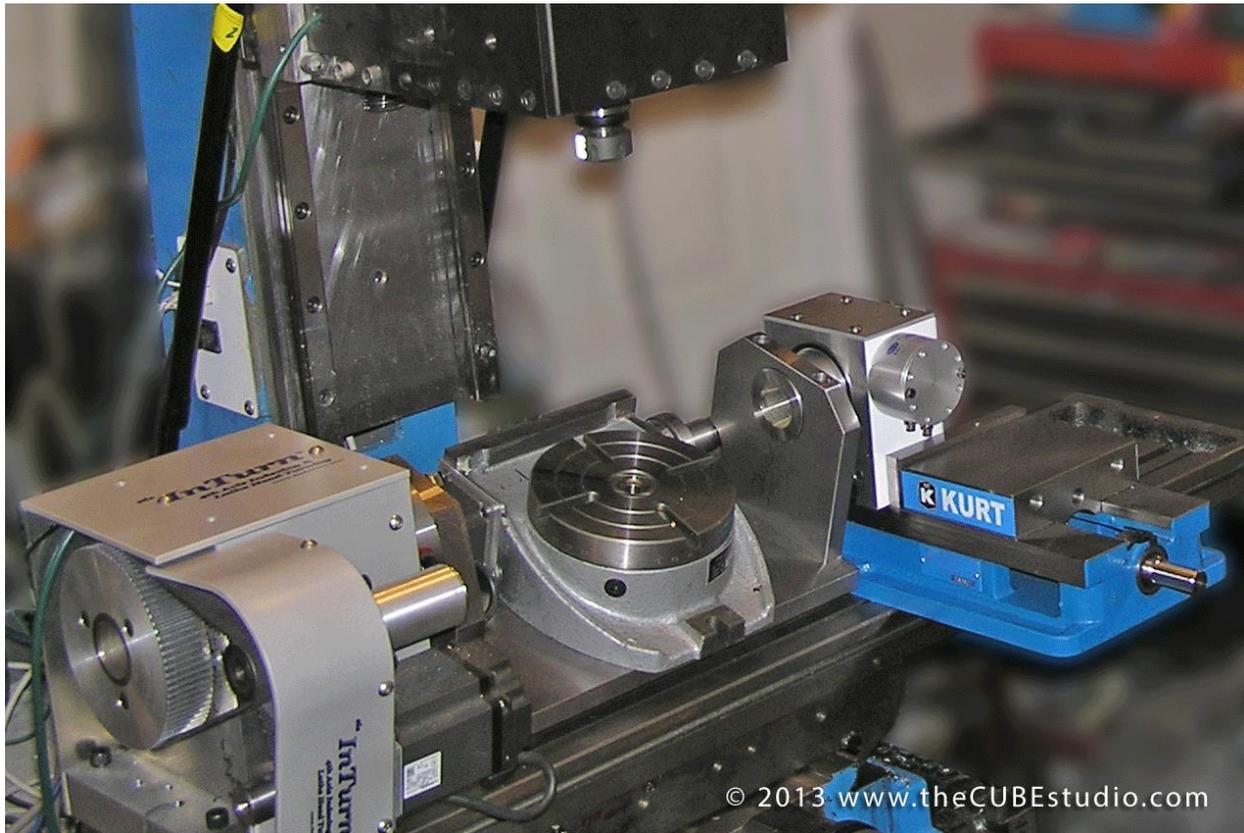
**The InTurn™ Tail Stock II is specifically designed to compliment the unique features of the InTurn™ 4<sup>th</sup> axis and provides multiple services;**
