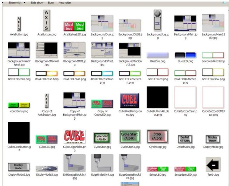
There is one exception to the folder naming convention used in the InTurn™ distribution. Copy the screen set **‘\InTurn\_Screenset\InTurn1920[suffix].set’** into **C:\Mach3**
