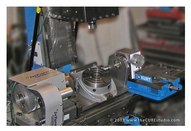
The InTurn<sup>™</sup> Tail Stock II is specifically designed to compliment the unique features of the InTurn<sup>™</sup> 4<sup>th</sup> axis and provides multiple services;
